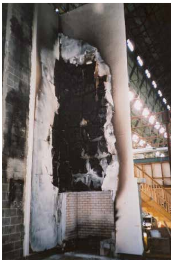
Figure 10: Thermosetting core without adequate fixings or fire breaks
