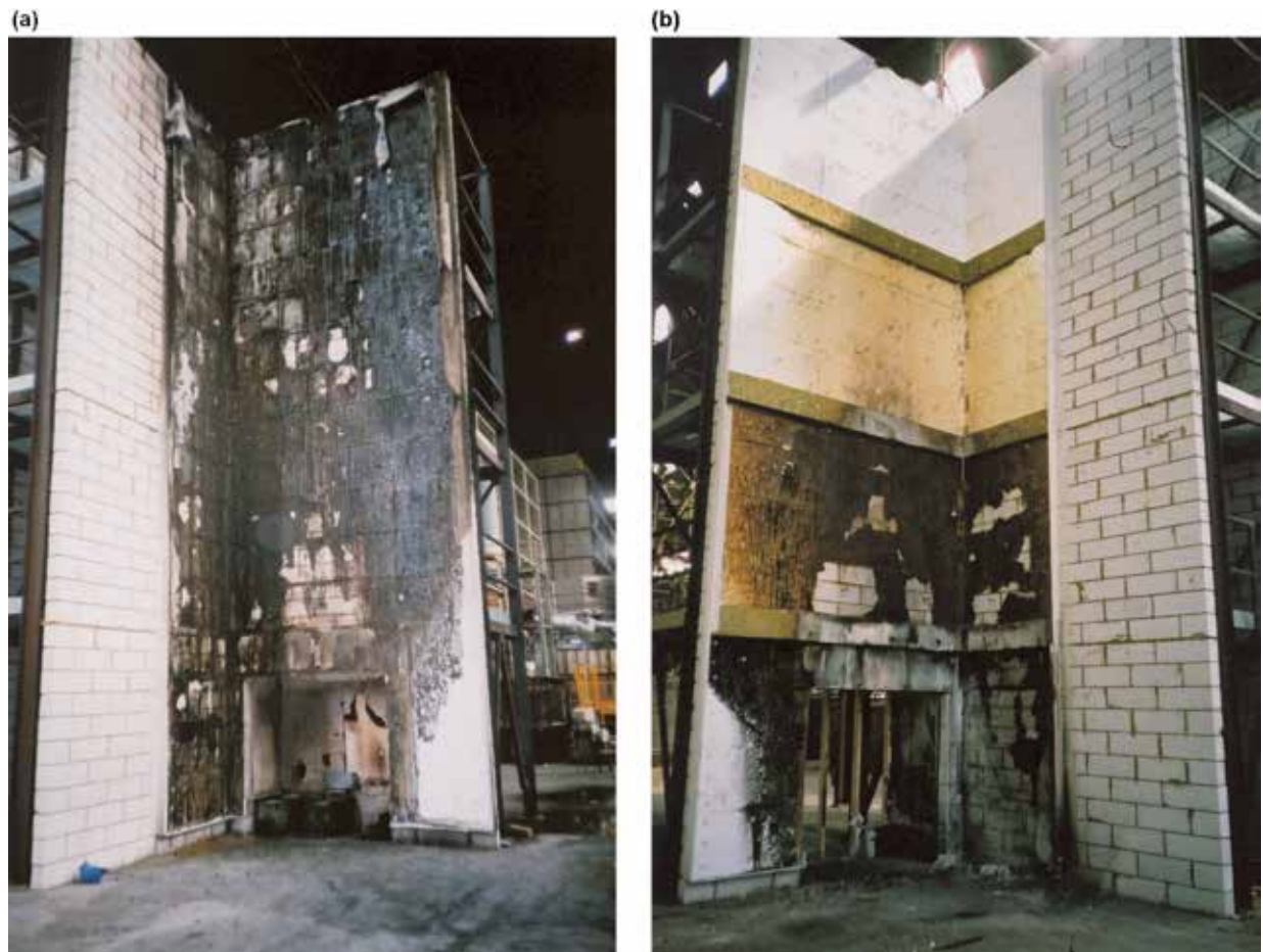
Figure 11: EPS system after test (a) without fire barriers, (b) with fire barriers
