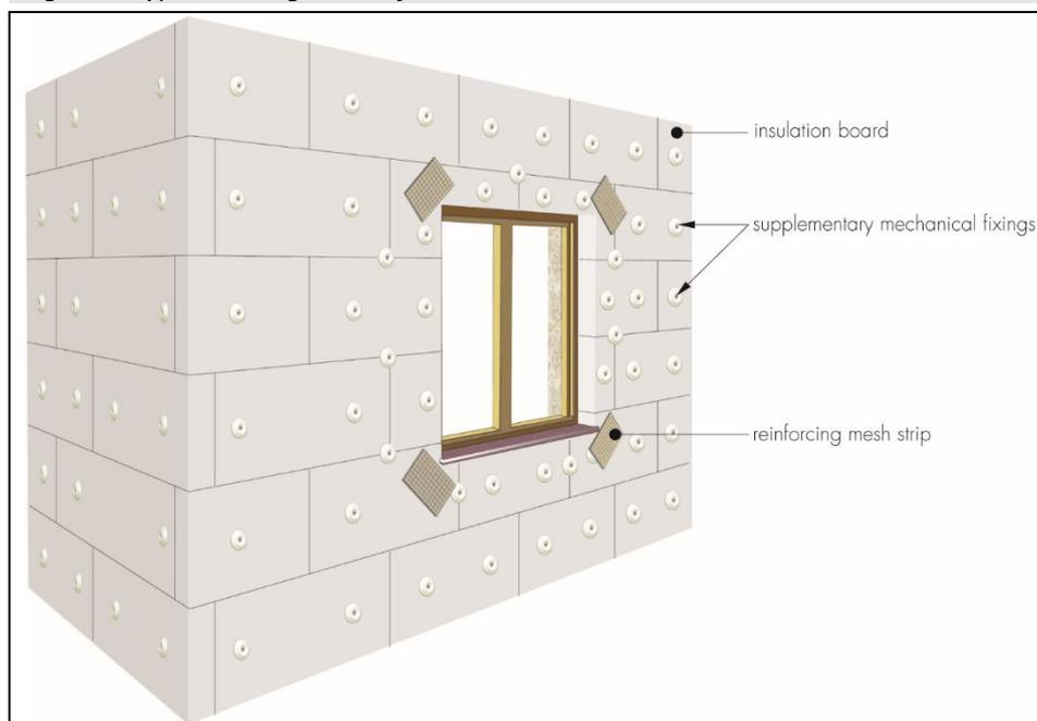
16.10 Prior to the application of the main reinforcing mesh, additional pieces of reinforcing mesh (approximate size 300 by 200 mm) should be used diagonally at the corners of openings and at window reveals (see Figure 5).
