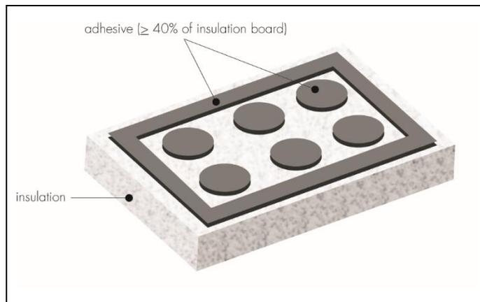
16.8 The first run of insulation boards is positioned on the base profile and pressed firmly against the wall. Care should be taken to ensure that all board edges are butted tightly together and alignment checked as work proceeds (to achieve a flush finish). Where existing render is on the wall or dubbing out render has been used, care should be taken when aligning the boards as the effective embedment will be reduced.
