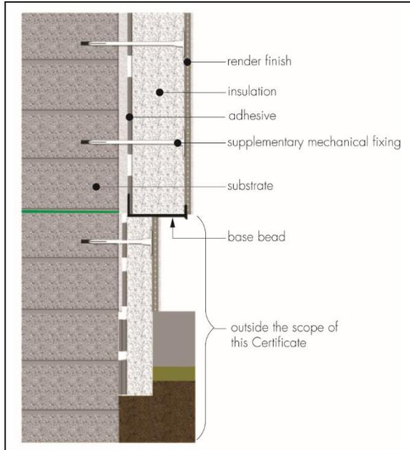
16.6 The adhesive is prepared by mixing each bag with the required amount of clean water in a suitable container as described in section 1.2, using a paddle drill mixer to create a paste-like mortar until the desired consistency is achieved. After allowing the adhesive to rest for 5 minutes, it is stirred again in accordance with the Certificate holder's instructions.
