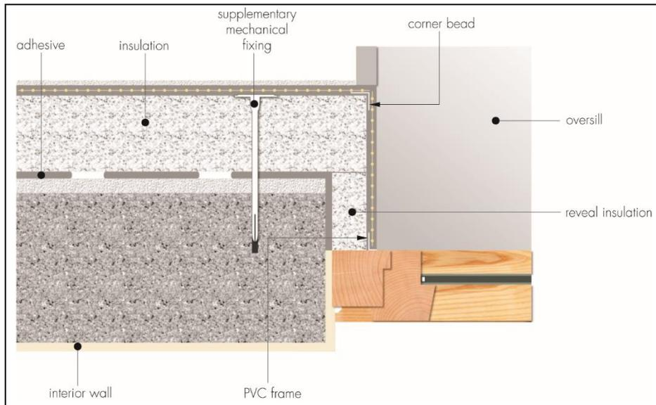
Figure 9 Window sill detail
